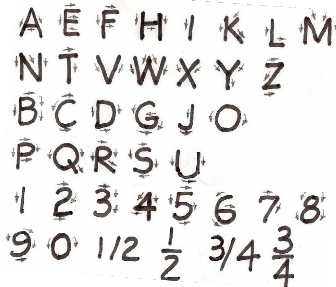
Fig. 3 Strokes for freehand lettering
